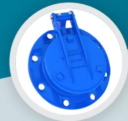
The valve has a body and bonnet in ductile cast iron EN-GJS-500-7 (GGG50) epoxy coated with 250 microns minimum thickness. The bonnet has a groove designed to fit a rubber sealing in EPDM (for water systems) or in NBR (for wastewater/sewage systems).
